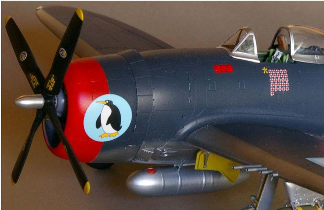
Since this is highly detailed "front office," I spent a lot of time painting the other individual pieces aluminum, black and olive drab according to my research photos. I finished off the cockpit with dots of red, silver and white on the handles protruding from the throttle, breaker boxes, etc.
