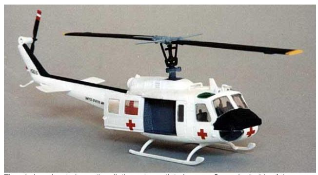
The windows located over the pilot's seats are tinted green. Spray the inside of the windows with a light coat of Tamiya "clear green" acrylic paint. Acrylic paint does not "fog" clear plastic parts as will some that are enamel or lacquer based. All of the clear parts can be attached using Johnson's "Future" acrylic floor wax. This product also will not attack clear plastic and dries invisible. Attach the tail and main rotors and the model is complete.
