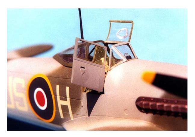
With the painting complete and dry, I sprayed Testor's Glosscoat over the model to get a smooth, glossy surface for the decals. The AeroMaster decals are thin and settle down into the engraved panel lines of the model with just a drop of setting solution. The decal sheet is complete with all of the necessary national markings and code lettering. A coat of Testors Dullcoat will seal the paint and decals.
