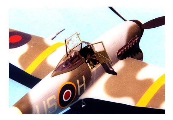
If your Typhoon is to carry bombs, be sure to open the bomb rack locating holes in the bottom of the wings then cement the wings together. The wing-to-fuselage fit is very good and no filler is necessary. The horizontal tail fit is just as good. The landing gear is next assembled and painted flat aluminum. The wheel wells are painted the same color as the cockpit interior.
