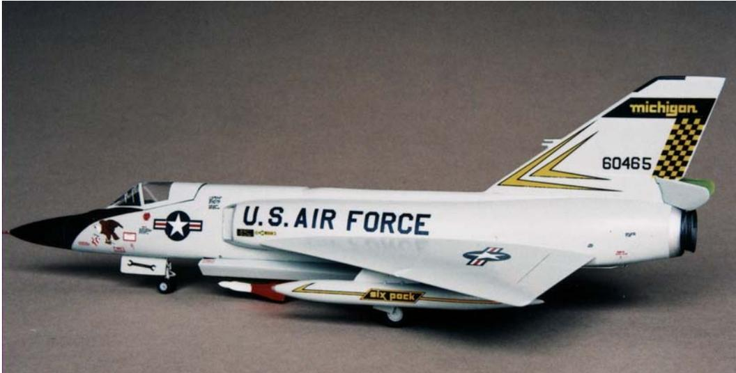
Glue the missiles to the launchers and set aside to dry. Assemble the wings and attach them to the fuselage. Filler is required at the wing-to-fuselage joint and on the vertical tail. Sand the entire airframe carefully to remove the rivet patterns and raised panel lines to achieve an overall smooth finish.
