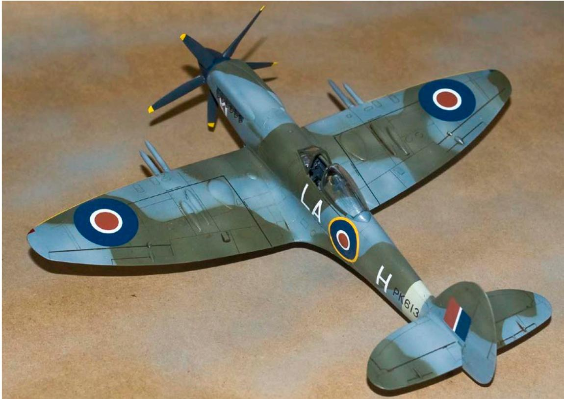
After modifying the interior parts, everything went together without any problems. The wings and tail planes fit well with just the normal cleanup of fuselage seam lines. I used cyanoacrylate and Mr. Surfacer.
